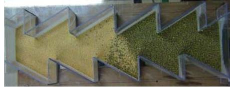
**FIGURE 3.** Axial segregation in an equal weight mixture of sarson (yellow) and moong (green). The vibration amplitude and frequency are 7 cm and 105 RPM, respectively.
