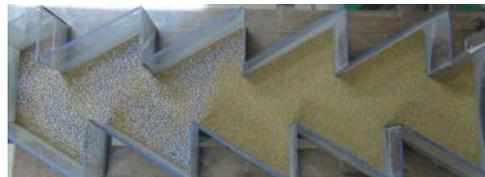
**FIGURE 4.** Axial segregation in a 1.75:1 weight mixture of steel balls and sarson. The vibration amplitude and frequency are 7 cm and 105 RPM, respectively.
